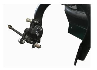
3.Install front wheel, crossing longer spacer pipe and spacer. Screwing nuts on the sides.
