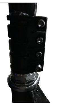
5. Assemble handlebar. Make two screws tightly.
