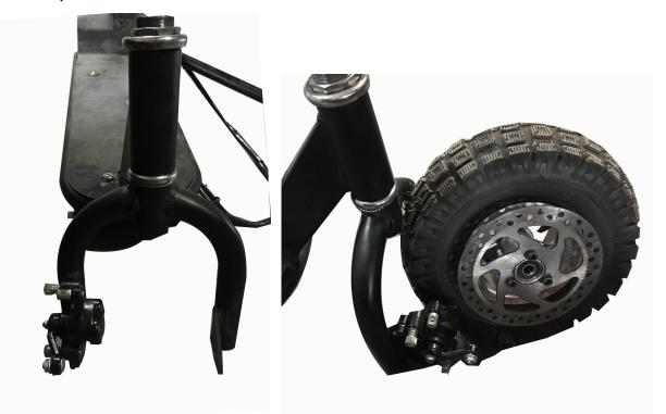
2. Cross axle from disc brake, put spacer and shorter spacer pipe.
