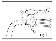
1. Insert two screws into the left and right handgrips (fig 1) .
