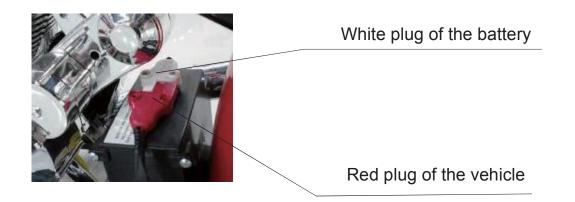
**IMPORTANT:** To prolong battery life, you must recharge the battery after each use. You must also charge your battery if it has not been used for 30 days or more.
