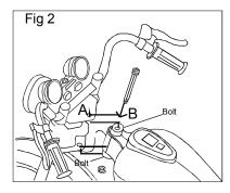
2. Connect the vehicle headlight wire to the corresponding body wire fig 3. Then align the holes in the front fork assembly with the holes in the vehicle body. Place the space rings, one on the top, one on the bottom. Then insert the hex bolt through the aligned holes, as shown in fig 2 and secure with the hex nut.
