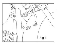
3. Locate the wires coming from the handlebar assembly and the bike and connect the terminals.
