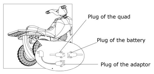
The red plugs for charging the battery are located under the right rear fender of the quad. Unplug the battery plug from the motor plug. Then connect the red charger plug into the battery plug, then plug charger into a household outlet. When the battery is fully charged unplug the charger and reconnect the battery plug to the motor plug.
