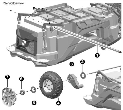
Cut off the plastic ties on the rear axle frames with a scissors. Release the gear boxes, but DO NOT disconnect the connectors of the gear boxes.
