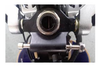
First remove the bolts and nuts and place the steering column upright on the upper plate of the column.
