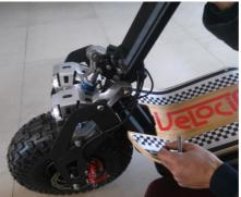
Attention:When installing the steering column, do not pull the cable too much to avoid damaging the cable and joint, causing failure.
