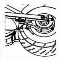
2 If the brake lever adjuster is threaded outward and the brake still has too much slack, use the back brake adjuster at the rear brake for additional adjustment.
