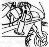
1 Remove valve extender/ adapter from right handgrip.
