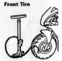
1 Using a bicycle-style tire pump equipped for a Schradertype valve, inflate the front tire to the PSI indicated on the sidewall of the tire.
