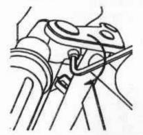
2 Using a 6mm hex key wrench, tighten both the left and right side handlebar clamps by turning the screws clockwise. When properly tightened, the handlebars cannot be twisted out of alignment.
