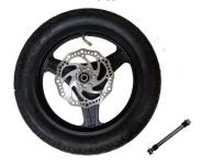
Insert the axle through the scooter frame and then the bushing . A bushing goes on each side of the wheel as a spacer between the wheel and the scooter frame. Tight the nuts on the axel to secure the wheel.
