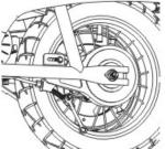
Right Side (Throttle) Safety hook 3/8 Axle locknut
