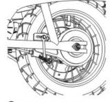
2 With two 8mm wrenches. loosen brake housing anchor and disconnect. Keep the spacer and washers together
