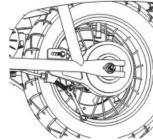
3 With a 10mm wrench, loosen the brake cable anchor and disconnect the cable.
