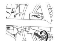
2 If brake is too tight or has too much slack, use a 10mm wrench to loosen the nut for additional adjustment on the brake cable on the rear wheel. Securely tighten nut when done.
