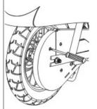
1 With a Phillips screwdriver, remove the screws that secure the chain guard. Remove chain
