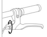
1 To adjust the play, thread the brake lever adjuster on the hand brake in or out 1/4 to 1/2 turn until the desired brake adjustment is attained. Most adjustments are complete at this step. If brake still needs further adjustment, proceed to step 2.
