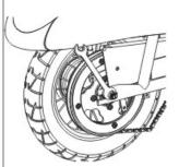
4 With two 15mm wrenches, loosen the axle. Slide the wheel forward to loosen the chain and remove the wheel. Note the sequence of the hardware. Note: Your hands will get greasy doing this.
