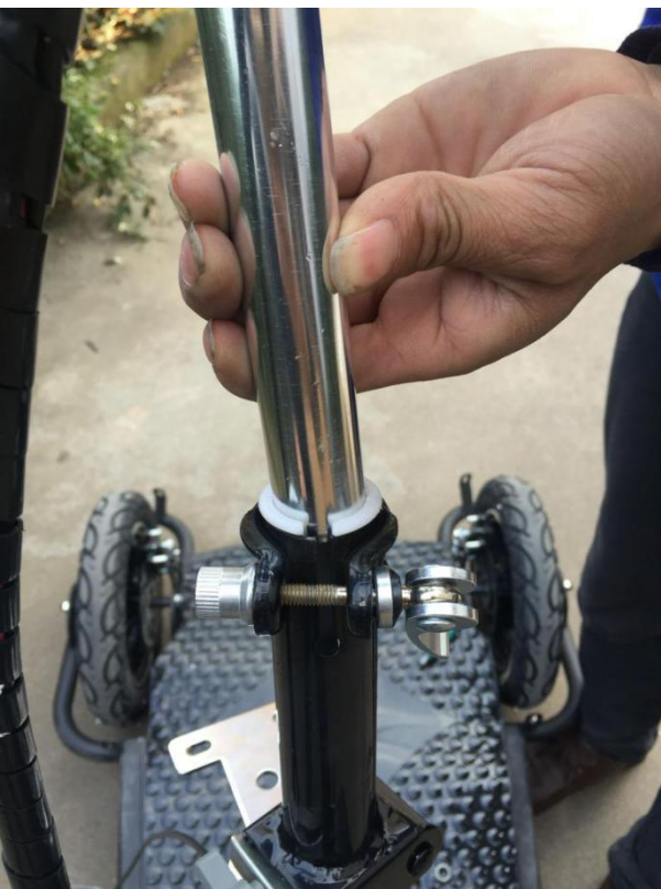
( 4 ) Install the pole, and screw the lock.
