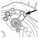
2 If the brake has too much slack, loosen the rear anchor bolt with a 5mm L-wrench and pull the brake wire tighter. The distance of the brake wire between the end of the cable and the anchor bolt should be between 37mm and 44 mm.
