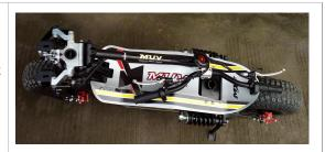
2. Unfold the scooter post and fasten the bolt.
