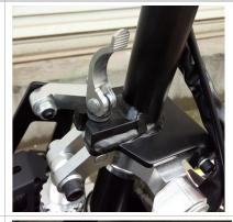
3. Attach the handlebar by inserting the silver handlebar clamp onto the handlebar post stopping just below the top. Be sure to orient the bars in the correct riding position with the throttle on the rider's right side. Secure the handlebars to the post by tightening the bolts on the clamp with the enclosed Allen wrench as shown.
