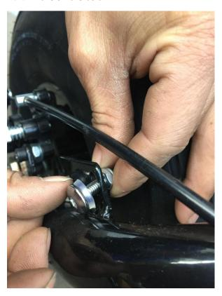
(2)Please note the position of the rubber washer, screw tight the bolt
