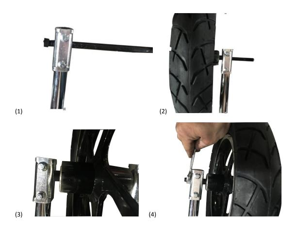
2. Install body. Use the axle across up and the body, and then put bearing and gasket. Next across down, put a gasket. Finally screw it. Check the screws tightly, pics(4).
