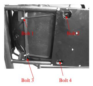
7) Place Solar panel on the rear of the Kart (above Battery compartment) Connect with the three bolts and washers as shown below.
