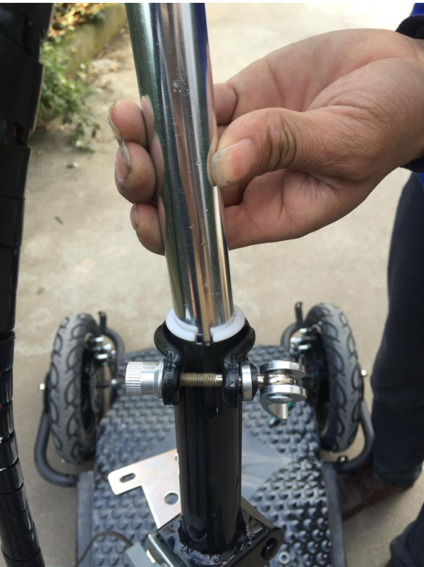
( 4 ) Install the pole, and screw the lock.
