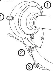
3. Fine Adjuster Feral - there are two on the front fork and it is important when adjusting the brakes that they are balanced to ensure even braking
