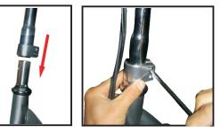
7. Adjust the brake by loosening the bolt on front brake wheel and pull the cable and retightening the bolt.
