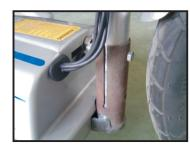
6.Ensure that the handlebar is facing front before tightening using the allen wrench provided.
