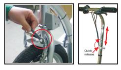
Note: Handlebar height can be adjusted by opening the quick release. Adjust handlebar to desired height and close quick release.
